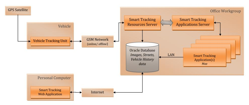
The Vehicle Tracking Units transmit their location packets to the "Resources Server" which is listening on a fixed IP address and port. The "Resources Server" logs the data into an Oracle Database and sends the information to the "Application Server", which in turn transmits the packets and violations to all connected Smart Tracking applications. Mainly the "Application Server" is responsible for updating all connected applications with the latest resource and task information.
